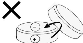
Fig. 2 stacked & jumble batteries
