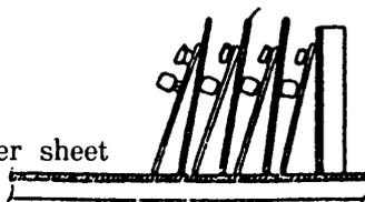
Batteries left on a work bench with positive and negative terminals in direct contact with the grounded rubber sheet cover are completely discharged.
